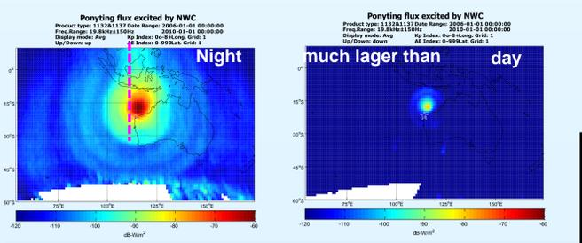
The energy attenuation is mainly in the earth-ionosphere wave-guide (0-65 km) and the D/E region of the lower ionosphere under 120 km. The energy would not change after penetrates the D/E region.
