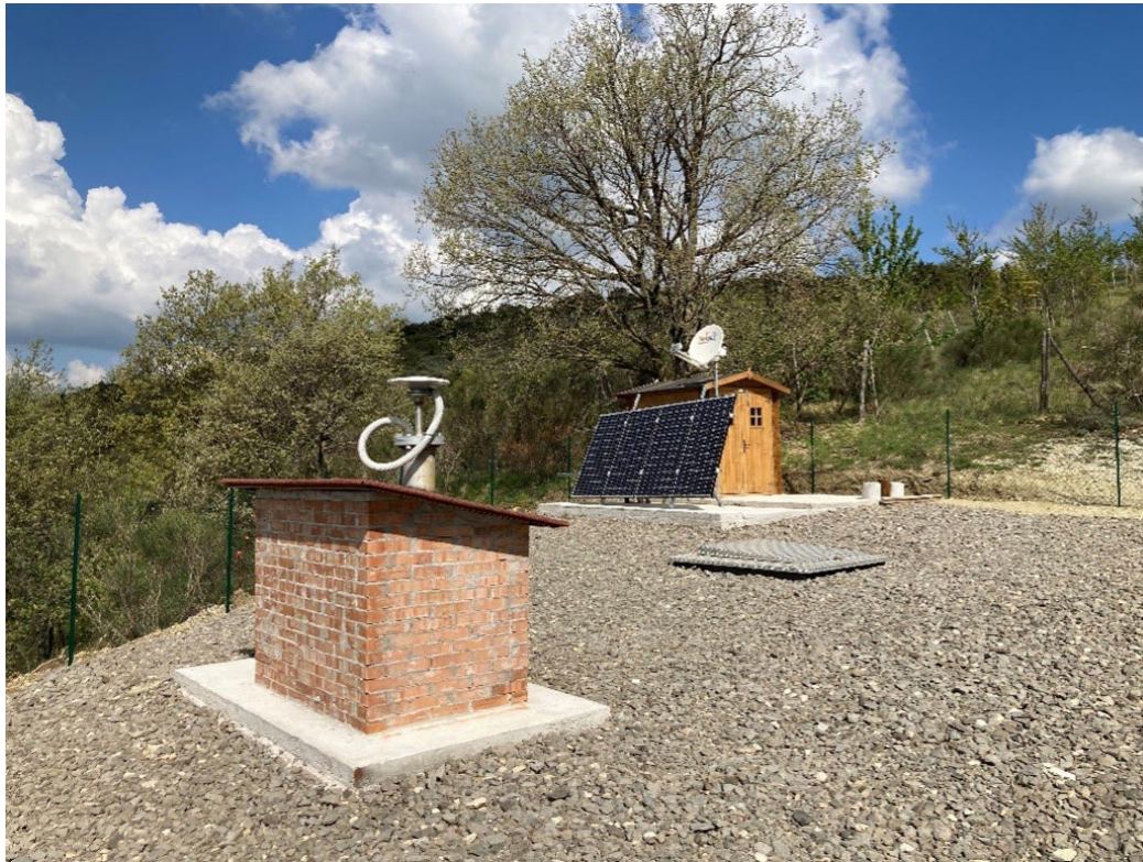
Figure 5. TSM2 observatory site: a single site hosting strain- and seismo-meters within a 160 m deep borehole, roundtrip fibre optic cable and pore pressure gauge within a pipe installed within the same hole. At the well head, covered by the small brick cottage (on the left), is visible the GNSS antenna, while in the centre of the picture there is the aluminium cover to protect the sensor pocket installed on the surface. On the right, the wood house hosting the acquisition and satellite transmission system with Meteo antennas on the roof. The power system composed by a set of solar panels are placed in the front of the house.
