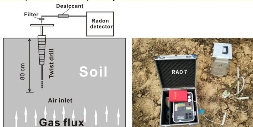
Fig. 2 Sampling scheme and instrument employed for soil gas Rn concentration measurement.
